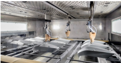
VEN SPRAY: A view of the spray coating booth with a special Multiflex rail system, which allows the four linear axes, each with two spray guns, to also move vertically during the horizontal stroke, i.e. in an arc shape adapted to the shape of the workpiece.
