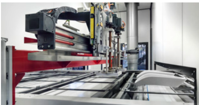
VEN CLEAN: Dust removal and ionization systems permit the removal of electrostatic charges, which promote the adhesion of dust on component surfaces.
